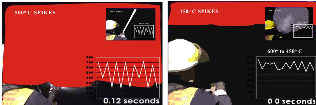
*Further effects of high temperature vapour expansion where 500°C spikes and 4000-1 vapour expansions force the smoke and thermal layers down into the lower regions of the room. The less severe 150°C spikes from the 3D fog pattern enable the smoke and thermal layers to rise as the contraction of the cooling gases counters the expansion of vapour at 2700-1*
