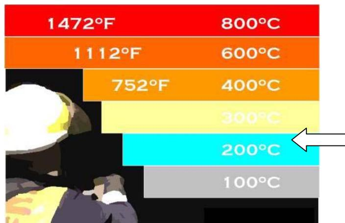
*Typical temperatures in a room fire (or adjacent room) bordering on flashover (arrow indicating one metre from floor)*
