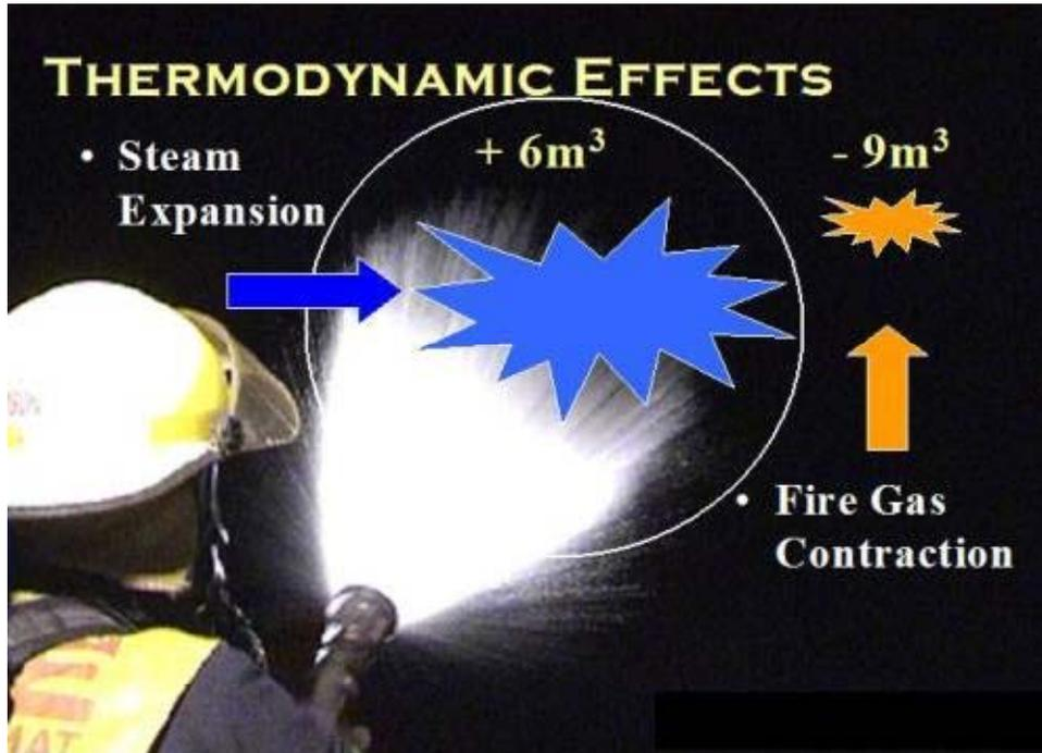
*An example of thermodynamic effects where the expanding water vapour is countered by fire gas contraction*
