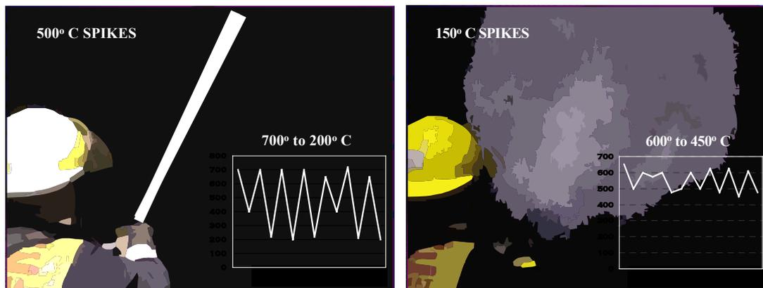
*In these computer-simulated images from real fire data, the effect of high temperature evaporation at the ceiling using a flow-rate of 360lpm can be seen in the 500°C spikes (left) from a straight stream when compared to the less severe 150°C spikes from the 3D water-fog pattern (right)*
