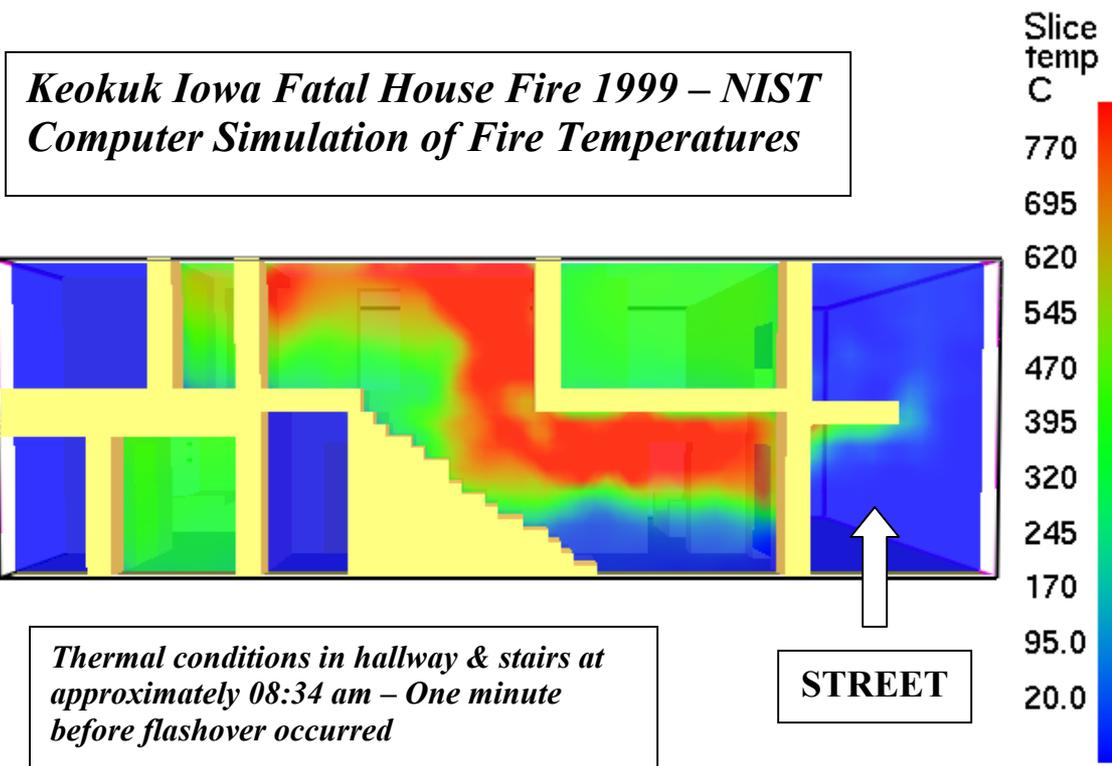
Typical temperatures that may be encountered pre-flashover in compartments adjacent to the fire compartment. Note temperatures close to 800°C at the ceiling and over 300°C at one metre from the floor. The classic warning sign of flaming in the overhead was most likely taking place in this situation, although the dark smoke at the ceiling may have masked it.
